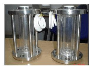
A sight glass consists of one glass pipe section, one metal frame, a pair of PTFE bushes and washers and an acrylic cover. Borosilicate pipe section is highly heat resistant, has excellent chemical resistance and has low thermal expansion. Metal frame is composed of two flanges which are welded with studs so that the stresses and vibrations of the pipeline do not transfer to the glass pipe section. Its check nut keeps the glass pipe section in compression and provides ease in replacement.
